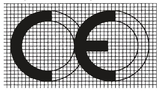
If the 'CE' marking is reduced or enlarged the proportions given in the graduated drawing set out in this point must be respected.
